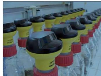
Figure 1 - Dispositif OxiTop® (ADEME 2012)
